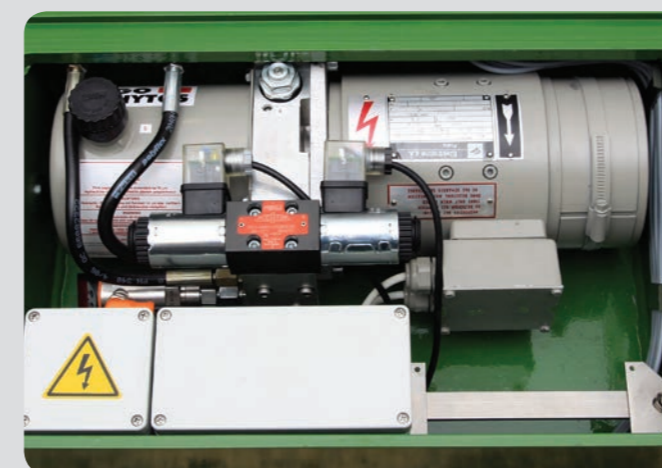
Elektroline compact 600-750 V DC electromotor
